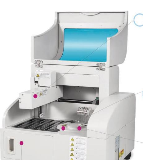
Unique discrete, X+Y+Z dispensing system Sample/Reagent probe with stirring function Automatic probe washing Liquid level detection Collision protection
