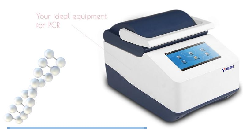
7 inch color LCD touch screen, no hard keys, functions quickly accessible through simple, one-touch commands
